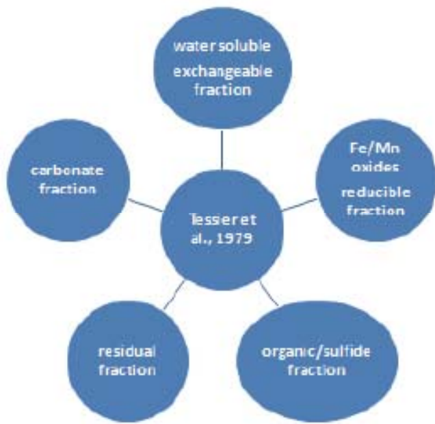
Figure 2: Fractionation of heavy metal (loid)s in the soil.
