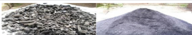
Figure 4: The state of charcoal before (left) and after (right) crushed. Source: Abewa, et al. [12].
