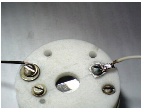
Figure 1: General view of the cassette for CEMS with a filamentous tungsten anode with a diameter of 25 microns.
